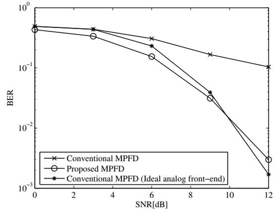
Figure 1: The BER performance versus SNR of the conventional and proposed MPFDs
