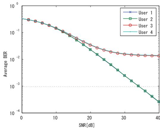
Fig. 3. The BER performance of the localized OFDMA
