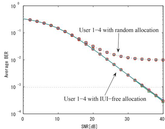
Fig. 4. The BER performance of the OFDMA with the random and IUI-free subcarrier allocation
