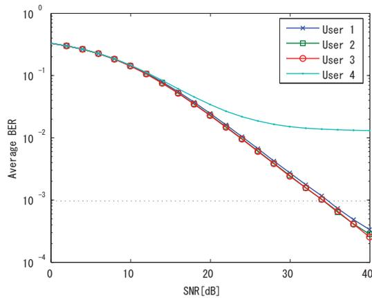
Fig. 2. The BER performance of the interleaved OFDMA with the conventional receiver
