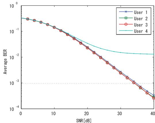
Fig. 2. The BER performance of the interleaved OFDMA with the conventional receiver
