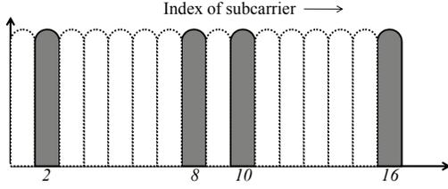
Fig. 1. Subcarrier allocation of the 2nd user in the proposed IUI free OFDMA where  $K = 4$  and  $M = 4$
