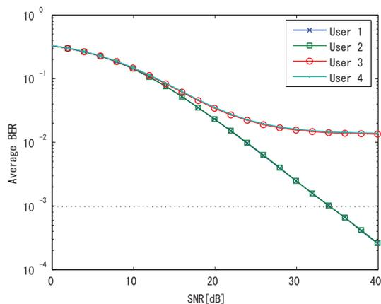
Fig. 3. The BER performance of the localized OFDMA
