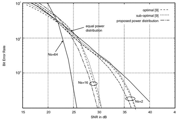
Fig. 5 BER performance for uncoded OFDM with 64-QAM
