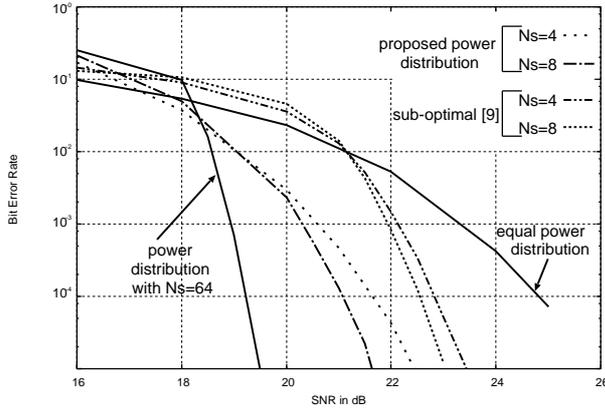
**Fig. 8** BER performance for coded OFDM with 16-QAM and  $R = 1/2$
