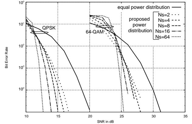
Fig. 6 BER performance of coded OFDM with  $R=1/2$  for QPSK and 64-QAM modulations
