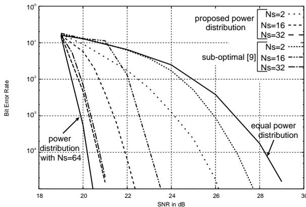
**Fig. 9** BER performance for coded OFDM with 16-QAM and  $R = 3/4$
