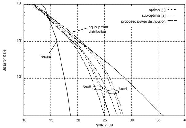
Fig. 4 BER performance for uncoded OFDM with 16-QAM
