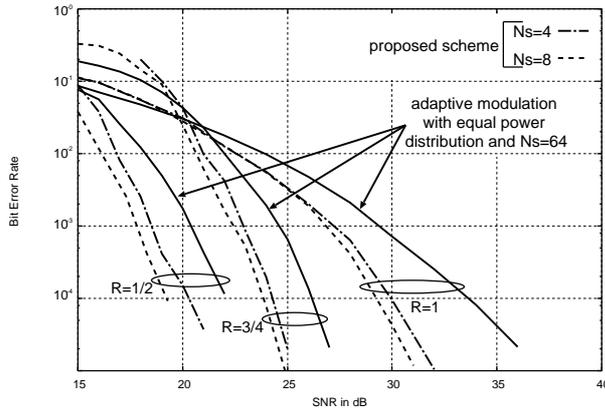
**Fig. 11** BER performance for uncoded and coded OFDM with  $\bar{B} = 3$
