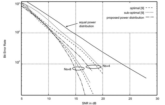
**Fig. 3** BER performance for uncoded OFDM with QPSK modulation
