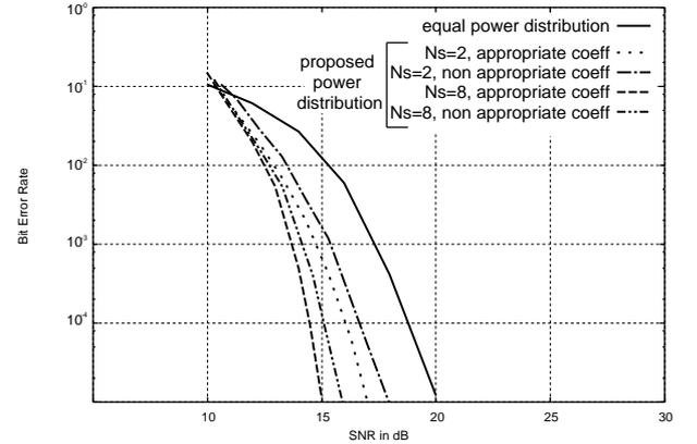
**Fig. 10** BER performance for coded OFDM with QPSK modulation using optimized and non-optimized  $a_m$  and  $b_m$
