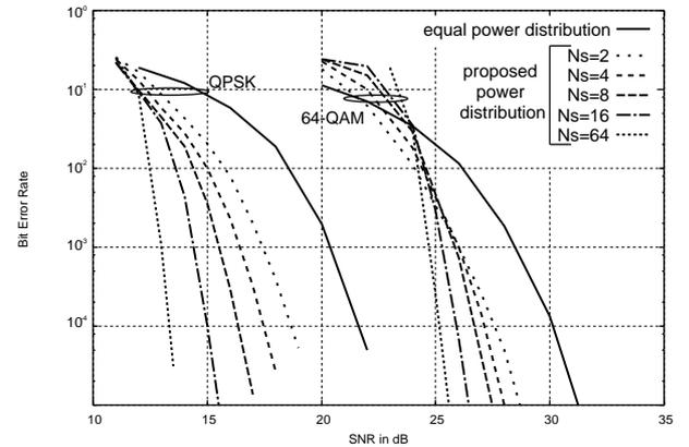
Fig. 7 BER performance of coded OFDM with  $R=3/4$  for QPSK and 64-QAM modulations
