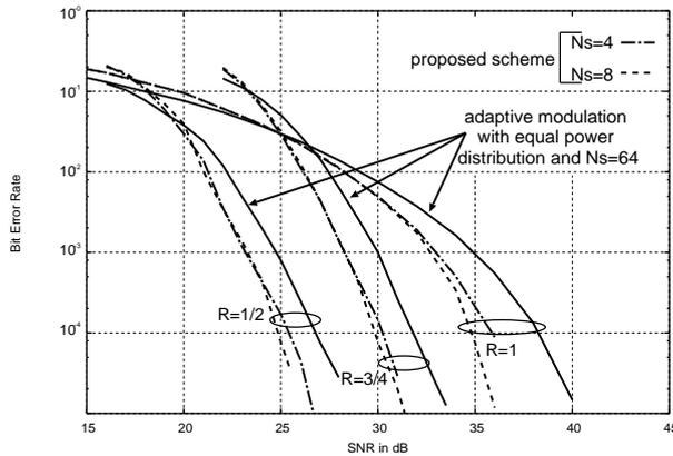
**Fig. 12** BER performance for uncoded and coded OFDM with  $\bar{B} = 5$
