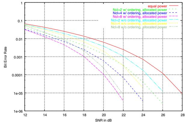
Figure 2: Performance Simulation for QPSK modulation
