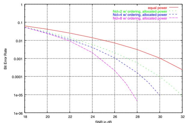
Figure 3: Performance Simulation for 16-QAM modulation
