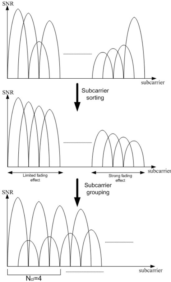
Figure 1: Principle of the group selection in function of the fading effect
