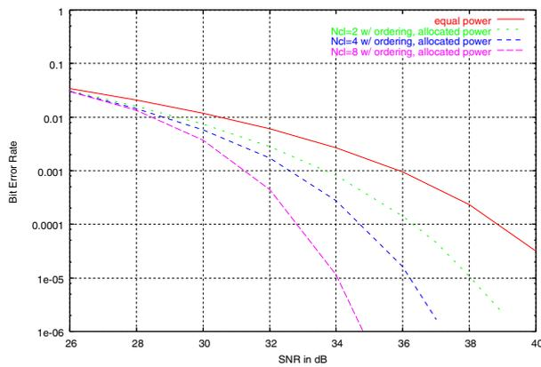
Figure 4: Performance Simulation for 64-QAM modulation
