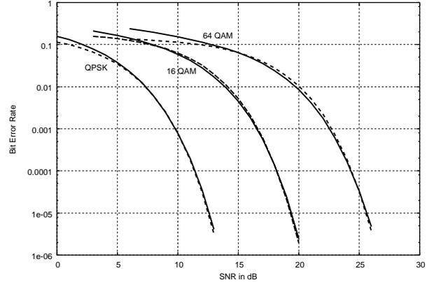
Fig. 1. Bit Error Rate for different modulations without channel coding (solid lines denote exact BER and dashed lines are fitting curves to the exact BER)
