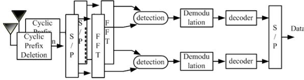
Fig. 3. MIMO-OFDM receiver scheme
